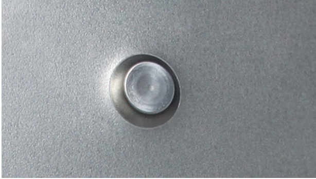
THE OUTCOME OF INSTALLING SELF-PIERCING RIVETS
