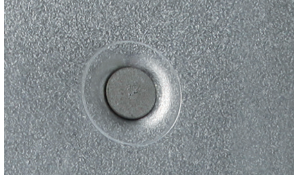
THE OUTCOME OF INSTALLING SELF-PIERCING RIVETS
