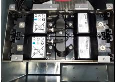
**79)** Insert the 6 grommets (20) in their place on the box (1). Route the machine DC harness (10), the charger DC harness (8) through them. Connect the Li battery – charger communication harness (7) and the Li battery machine communication harness (9) to the batteries
