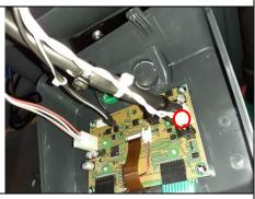
63) Stick it around the Ibutton-cable from the back side of the I-button reader. Clean the surface of I-button reader with brake cleaner or isopropyl alcohol
