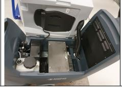
**90)** If the machine doesn't switch on, open the recovery tank, pick up the lid (2) and look at the LED on the battery. If it is blinking and becomes green then it is OK. If not, press the ON/OFF button of the Li-ion battery for about 5s and wait until the LED becomes continuous green. (See the manual (35))
