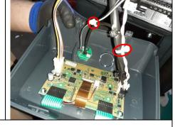
70) Tighten these wires to the metal side of the Italsea main control board with a cable tie
