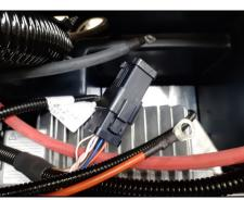
73) Connect a Control Cable (Nilfisk p/n: 106445009) between the 2 battery modules
