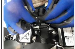
**78)** Prepare 1 positive braided cable (Nilfisk p/n: **106445008)** and 1 negative braided cable (Nilfisk p/n: **106445007**) and route the red cables to the + poles and the black cables (from the machine DC harness (10) and the charger DC harness (8)) to the – poles of the battery pack
