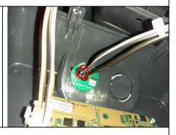
64) Grab the twisted pink-white CAN wire and the wire of the Reed switch of the Li battery machine communication harness (9) and push them through the hole ...
