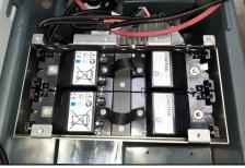
**77)** Since the standard KIT doesn't contain the TC1 module, connect the dummy, separate ITT CANNON male plug to the wired ITT CANNON female plug of the Li battery–machine communication harness (9)
