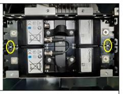
72) Insert 1 or 2 (depends on the customer's demand) Varta 24V Li-ion batteries (Nilfisk p/n: 106479002) in the box
