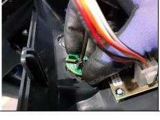
68) Connect the black connector of this harness (9) to the Reed switch PCB (25) (red)
