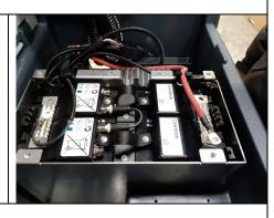
**74)** The connected Control Cable and the batteries in the metal box
