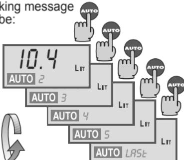
To confirm a PRESET value **press and hold down the AUTO key** until the METER displays:
