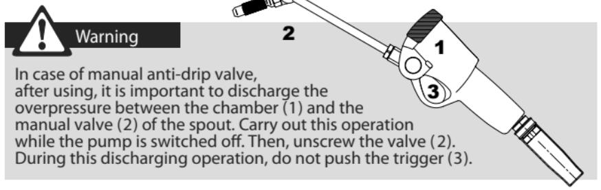
In case of manual anti-drip valve, after using, it is important to discharge the overpressure between the chamber (1) and the manual valve (2) of the spout. Carry out this operation while the pump is switched off. Then, unscrew the valve (2). During this discharging operation, do not push the trigger (3).
