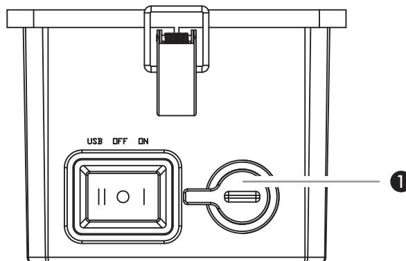
To switch the light on set the switch to the "I" (ON) position. To switch it off, set the switch to the middle position, "O" (OFF).
