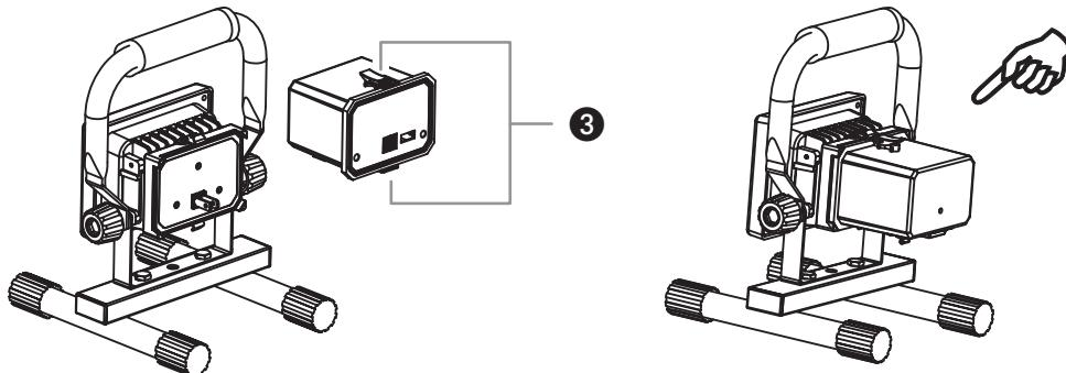
The battery is quick and easy to replace. Simply open the two fasteners ③ at the top and bottom, see drawing. This makes it possible, for instance, to charge the battery while continuing to work with the replacement battery (available separately).
